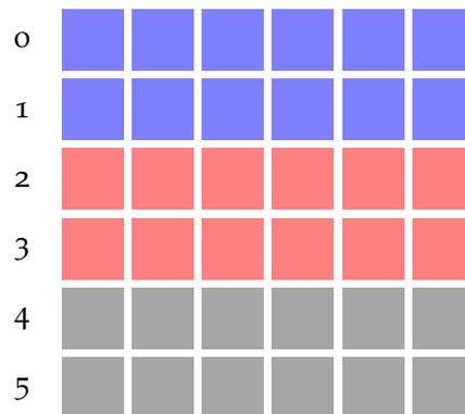
Figure 5: Row-wise distribution pattern of a matrix  $\mathbf{A} \in R^{6 \times 6}$  using 3 MPI ranks.
